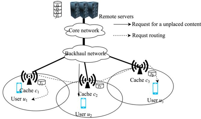
**Fig. 1.** Illustration of the unreliable network environment consisting of remote servers and edge nodes.
